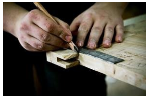
Measuring and marking out
