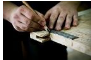
Measuring and marking out
