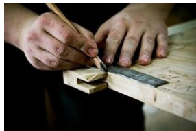
Measuring and marking out
