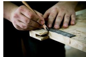
Measuring and marking out
